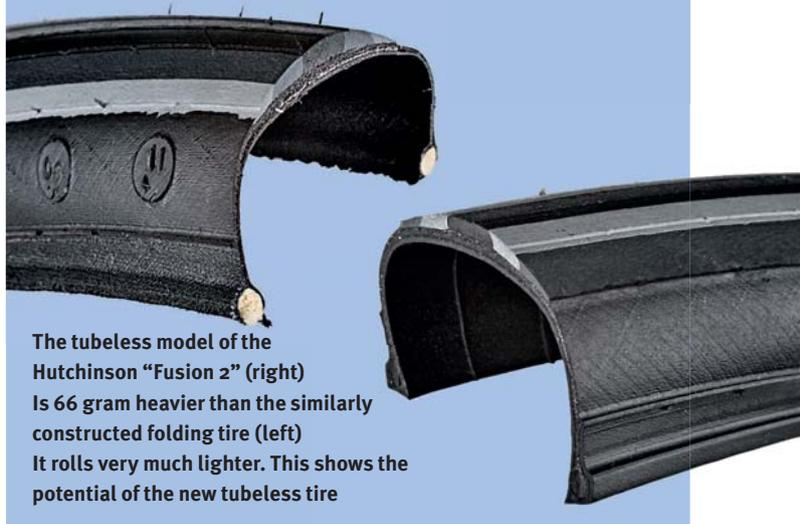
The tubeless model of the Hutchinson “Fusion 2” (right) is 66 gram heavier than the similarly constructed folding tire (left) It rolls very much lighter. This shows the potential of the new tubeless tire
