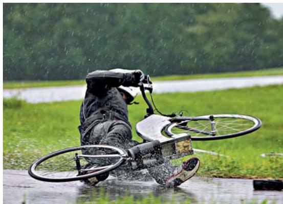
good tires show by the response from the front wheel where the borderline begins. They start to drift and sputter. This can be controlled by the rider's smooth reactions. On extreme, slippery surfaces the differences between an adhesive mixture and a normal rubber top disappear. The back wheel usually slides out which nearly always leads to a fall. It is difficult to judge a road surface ahead, especially if the
