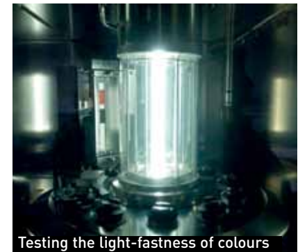
Testing the light-fastness of colours
